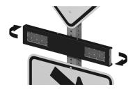
Rotate the light bar towards the incoming vehicle lane, independent of the wire hole location.
